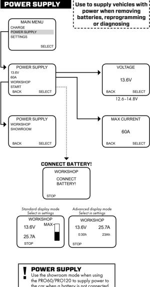
Use the showroom mode when using the PRO60/PRO120 to supply power to the car when a battery is not connected. Spark protection is disabled when showroom mode is chosen. When using supply mode with a battery present, use the workshop mode.
